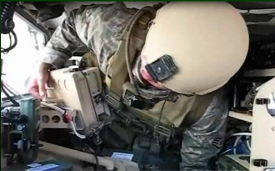
Screenshot from an AFOTEC video demonstrating that a forward combat air controller in combat gear could not exit a High Mobility Multipurpose Military Vehicle with the Tactical Air Control Party-Modernization Vehicular Communication System installed. (Image courtesy AFOTEC).
