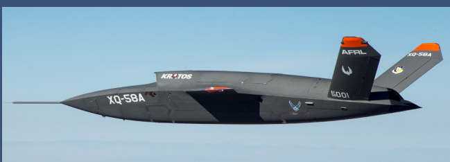
XQ-58A Valkyrie demonstrator first flight as part of the Skyborg program. (U.S. Air Force photo)
